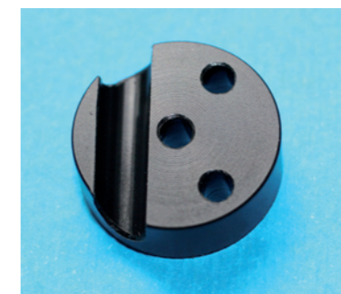
Figure 6. Plastic clamp with angled holes (Mickey Mouse type).
